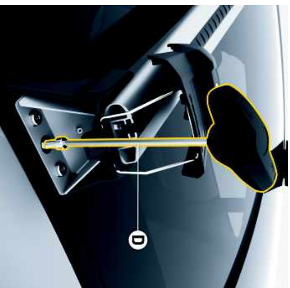
Fig. 171: Fold down the cover flaps and lock
