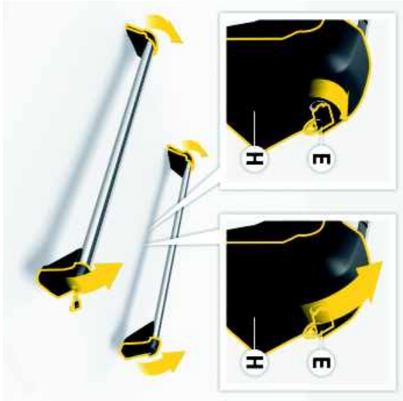
Fig. 162: Locking and folding up the cover flaps
