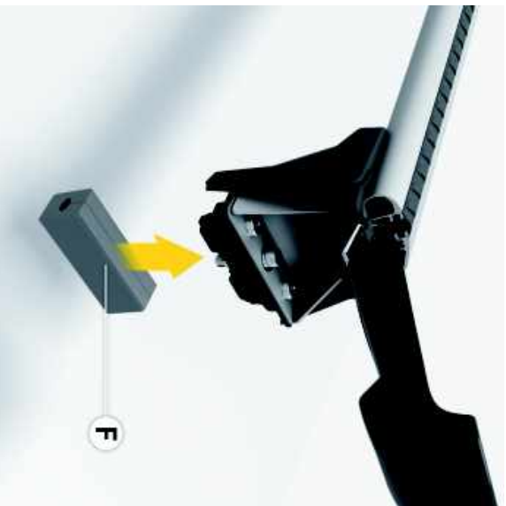
Fig. 168: Affix assembly protection
