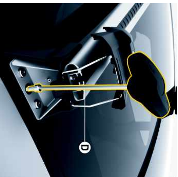
Fig. 166: Tighten fastening screws.
