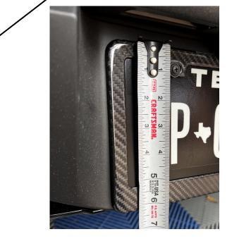
Raised plate in holder will protrude only 1" below this line and only over width of plate (12")
