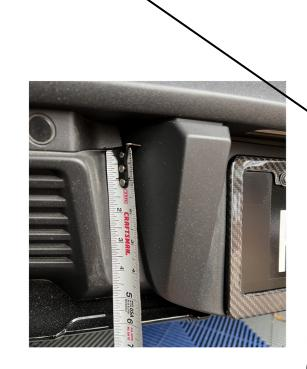
Picture of new plate holder (transparent) overlain on current US std. base plate holder to show positioning
