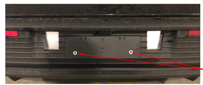
Goal to cover the large holes used to position/stabilize the US plate holder base.
