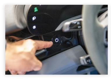
The power button is located left of the steering column. Press to turn on the vehicle.
