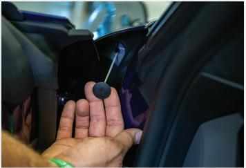
Pull the release towards the back of the vehicle.
