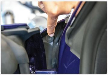
The release can be found on the inside of either the driver's side or the passenger's side door.
